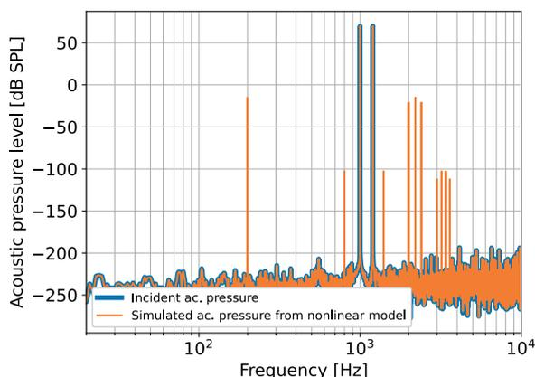
Figure 4: Theoretical spectra of the incident acoustic pressure (thick line) and of the acoustic pressure given by the nonlinear microphone model (thin line) for the 2-component measurement scenario
