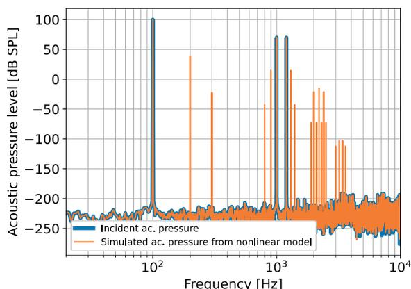
Figure 5: Theoretical spectra of the incident acoustic pressure (thick line) and of the acoustic pressure given by the nonlinear microphone model (thin line) for the 3-component measurement scenario
