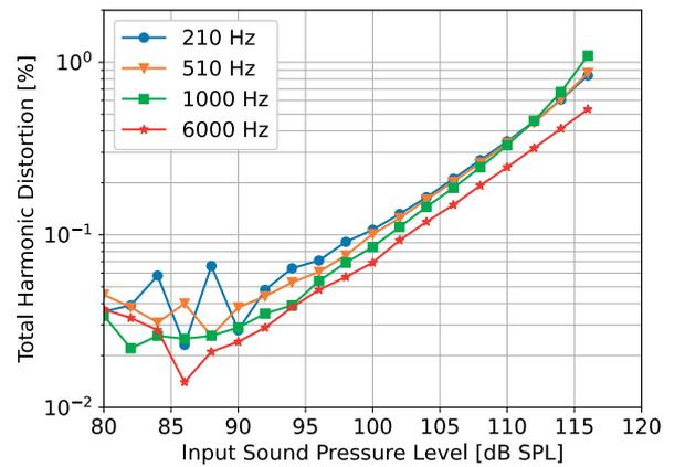
Figure 2: Measured Total Harmonic Distortion (THD) vs. input acoustic pressure level at different frequencies
