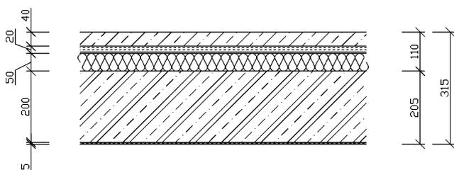
Figure 1: Configuration of a measured floating floor system
