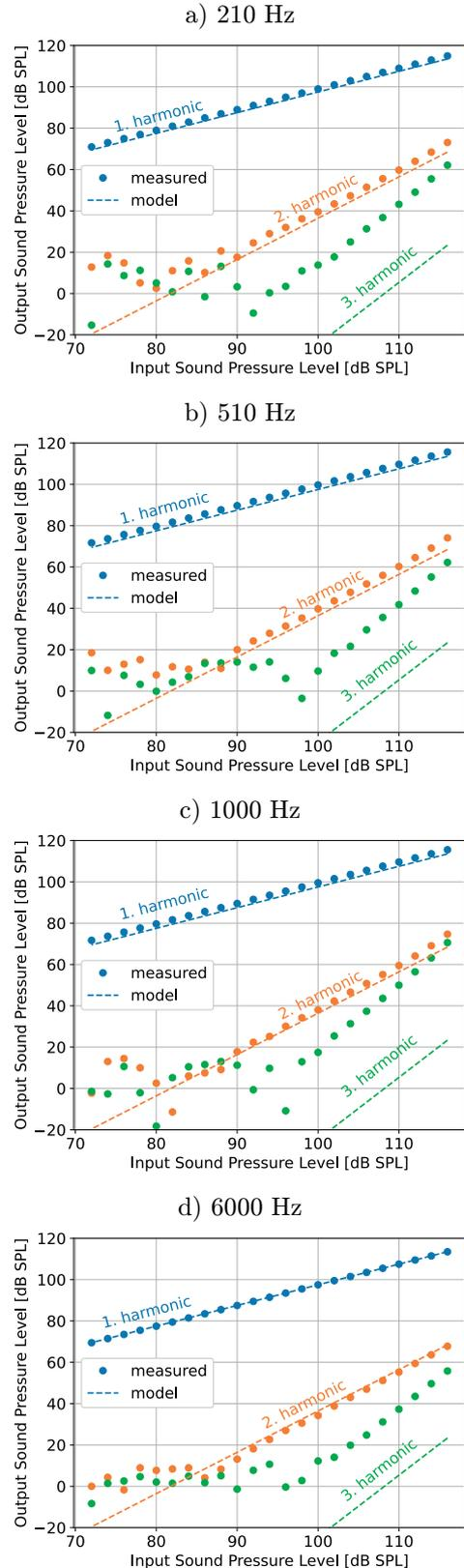
Figure 3: Measured (points) and theoretical (dashed lines) harmonics of the microphone under test at a) 210 Hz, b) 510 Hz, c) 1000 Hz, and d) 6000 Hz
